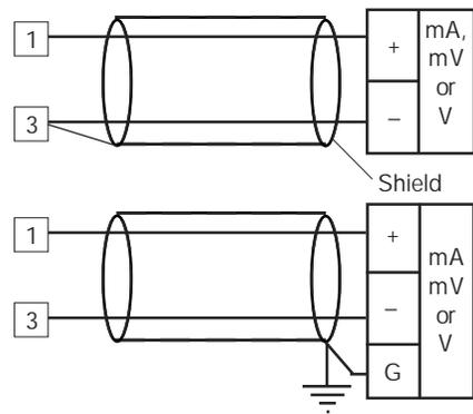
Fig. 6 mA, mV AND V INPUTS WIRING
