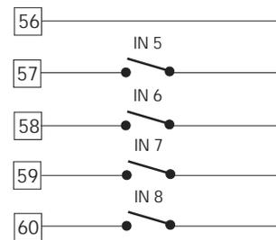
Fig. 9.C - LOGIC INPUTS IN 5, 6, 7 and 8 WIRING
