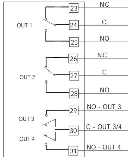
Fig. 11.A RELAY OUTPUTS 1,2,3 and 4 WIRING
