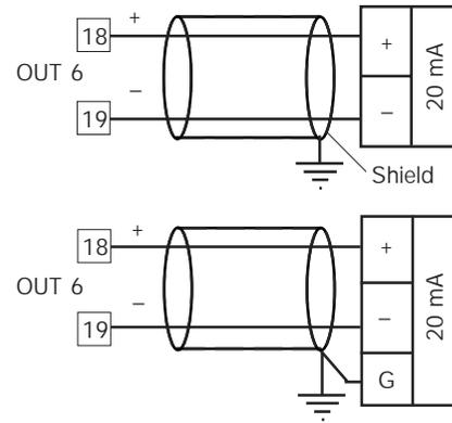
Fig. 16.B OUTPUT 6 WIRING
