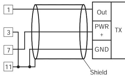
Fig. 7.B INPUTS WIRING FOR 3-WIRE TRANSMITTER
