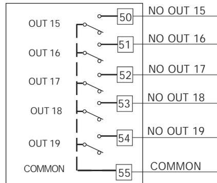
Fig. 11.C RELAY OUTPUTS 15 to 19 WIRING
