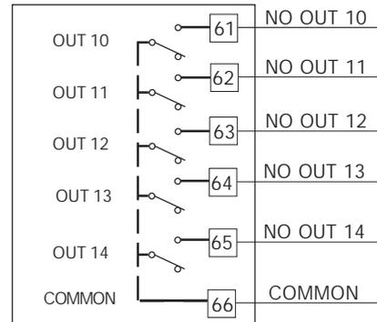
Fig. 11.B RELAY OUTPUTS 10 to 14 WIRING
