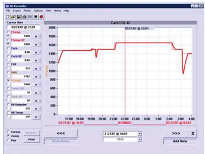
Fig. 4. Furnace chart displaying control with an intact radiant tube
