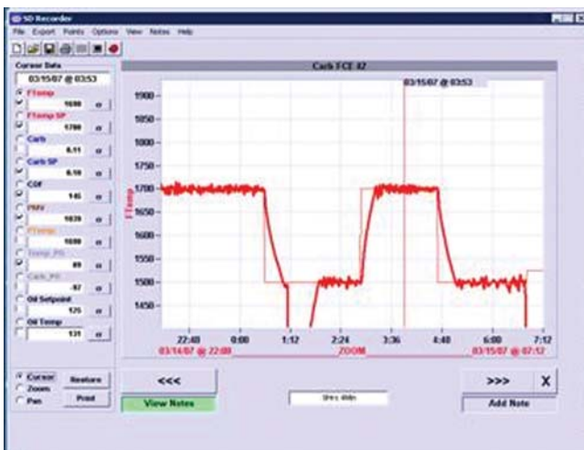
Fig. 3. Furnace chart displaying control with a cracked radiant tube
