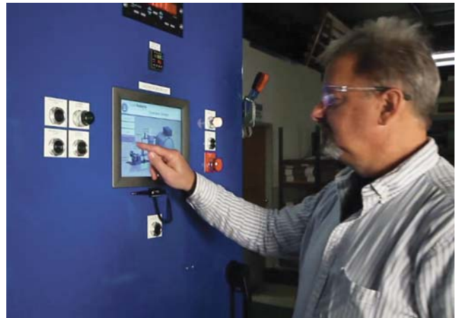
Fig. 2. An operator uses a customized human-machine interface (HMI) designed to control furnace functions as part of a plant supervisory control and data acquisition (SCADA) system.
