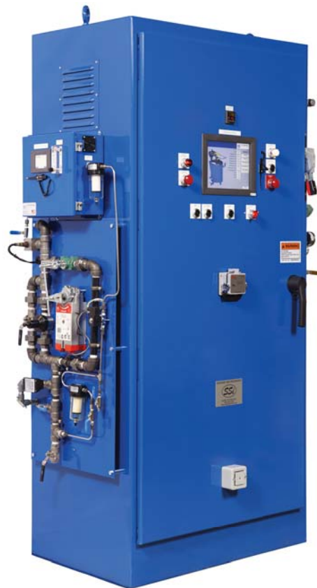
Fig. 3. A nitriding/ferritic nitrocarburizing (FNC) panel with specialized control equipment
